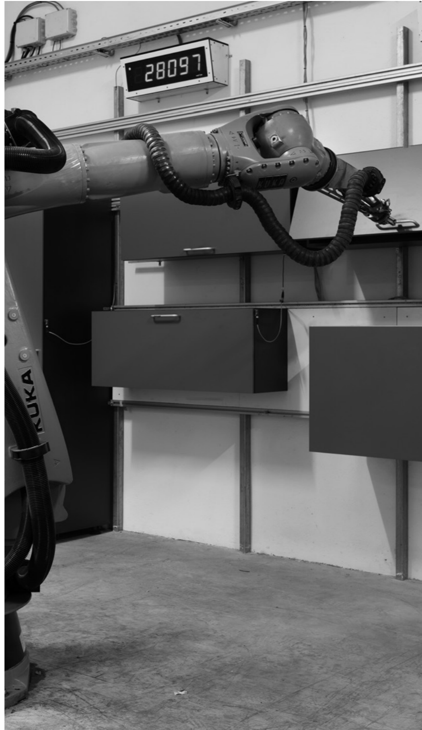
Robot-assisted test for opening and closing cycles.
